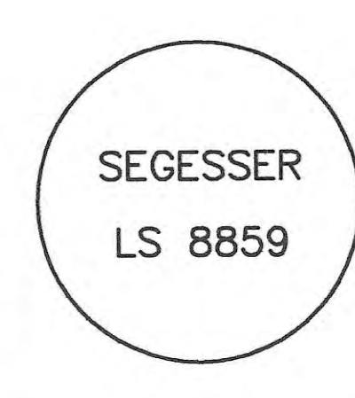
Typical Plastic Cap on set 5/8" Rebar
