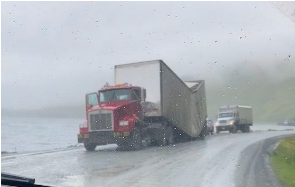
Figure 3: Pacific Stevedoring Truck with Chassis Failure due to Excessive Wear from Poor Conditions along Captains Bay Road, Fall 2021 (photo courtesy of Darin Nicholson)
