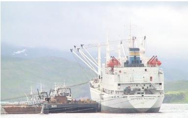
LIGHT CARGO DOCK, BARGE, TRAMPER BARGE IS BEING USED AS A "SPACER" TO PROVIDE DEPTH FOR TRAMPER
