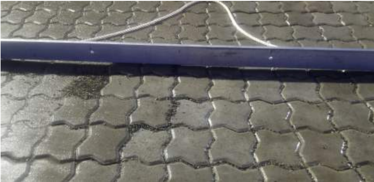
Paver blocks exceed allowable height tolerance
