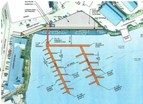
Proposed Concept (right) Side Tie: 218 feet Slips: 22—26 foot, 13 - 32 foot, & 20 42 foot
