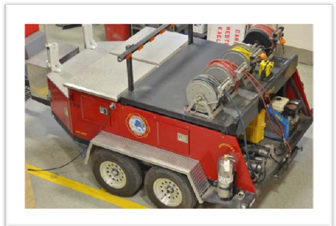
Figure 4: Mobile air compressor, attached here to equipment truck
