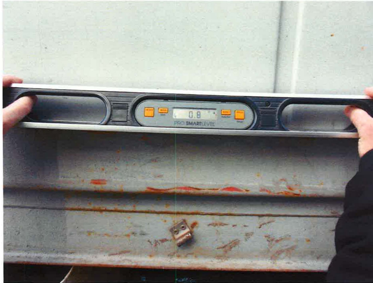
Picture of Horizon Lines Peterbuilt tractor – elevation angle from front of chassis to rear of chassis connected Bartlett fifth wheel in lowest position = 0.8 degree
