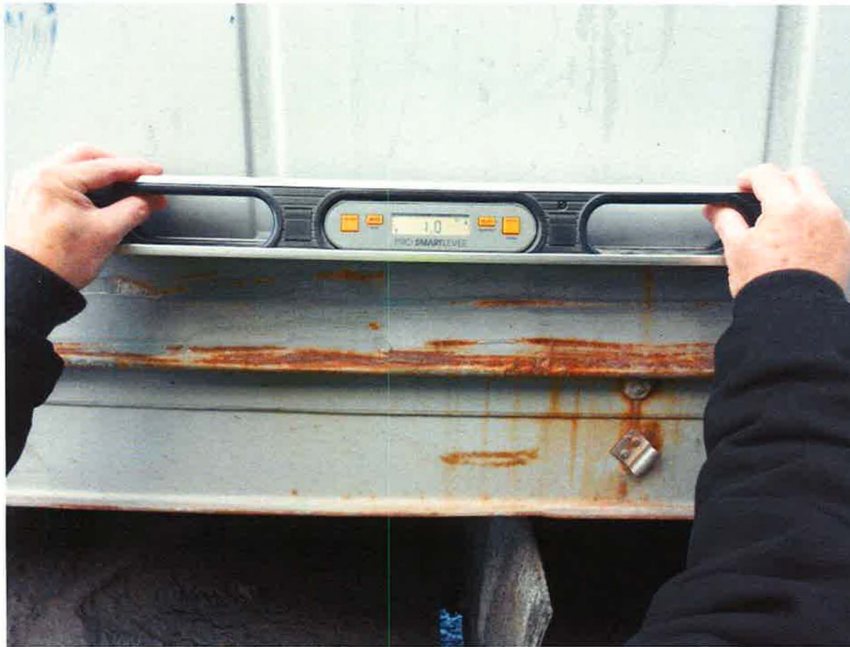
Horizon Lines Volvo tractor – elevation angle from front of the chassis to rear of the chassis, connected a Bartlett fifth wheel in lowest position = 1.0 degree.
