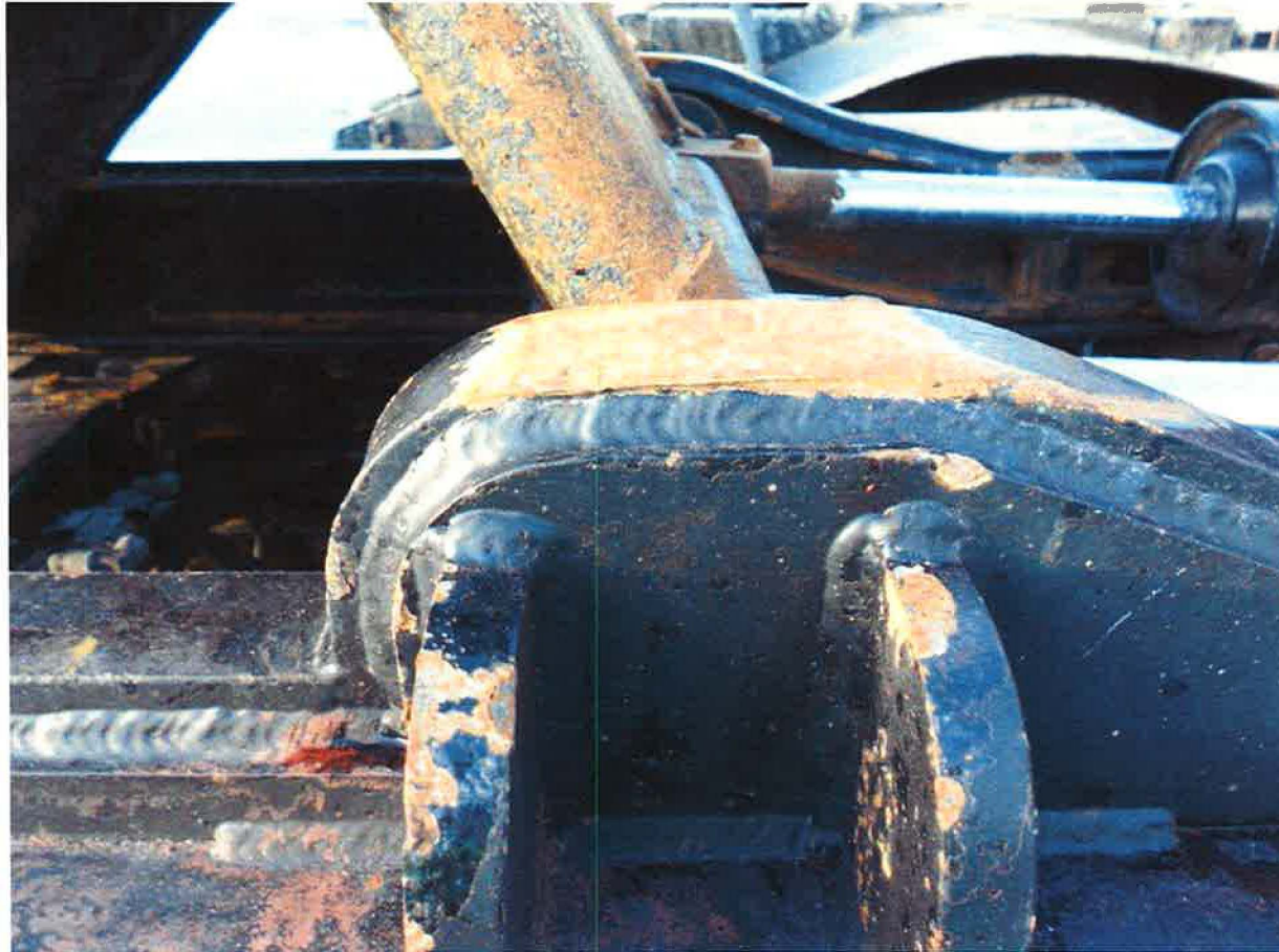
Damage to main frame from fifth wheel plate riding on main frame from a different angle.
