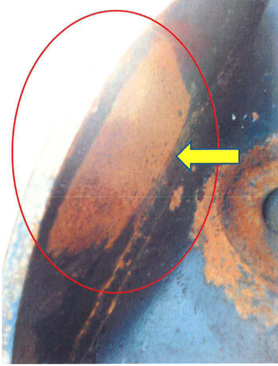
Bottom of fifth wheel plate getting worn away from main frame.
