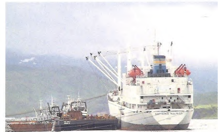
LIGHT CARGO DOCK, BARGE, TRAMPER BARGE IS BEING USED AS A "SPACER" TO PROVIDE DEPTH FOR TRAMPER
