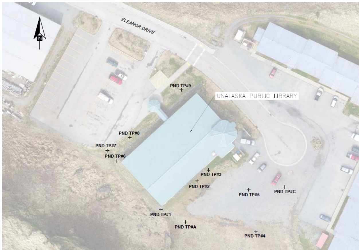
Figure 3-1. As-Built Borehole Locations
