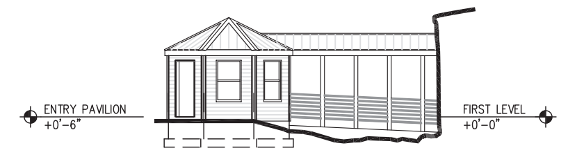
C5 ENTRY PAVILION - WEST ELEVATION - ADDITIVE ALTERNATE 1 - APPROXIMATE SCALE: 1/8"=1'-0"
