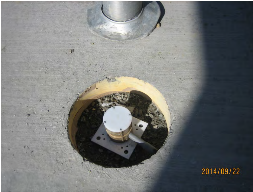
Temperature sensor near flagpole. Gray PVC conduit at sensor runs to junction box.
