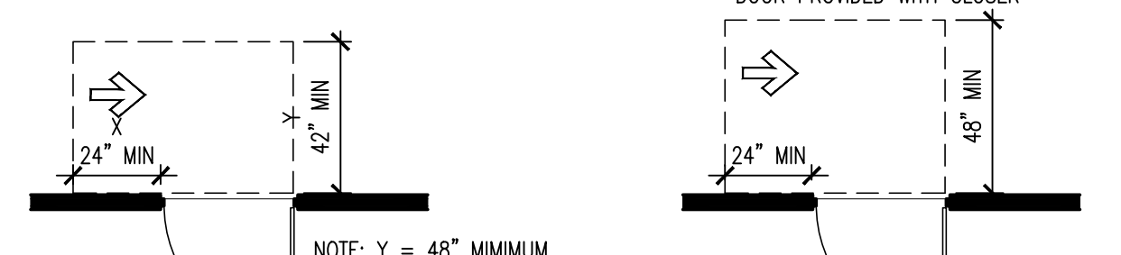
FIGURE 404.2.4.1 MANEUVERING CLEARANCES AT RECESSED DOORS AND GATES
