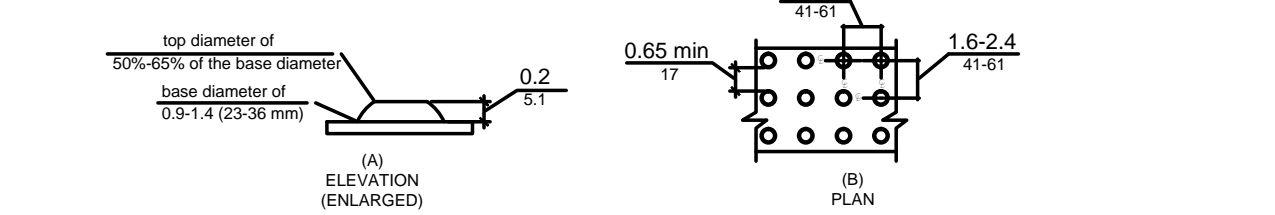
FIGURE 703.7.2 SIZE AND SPACING OF TRUNCATED DOMES
