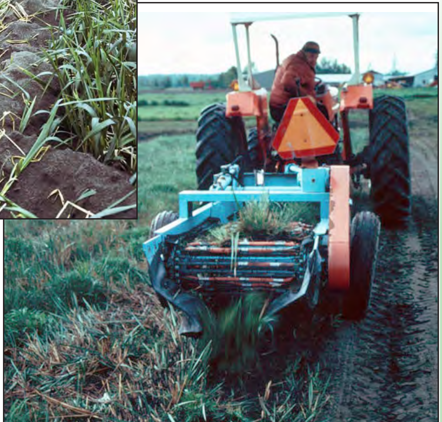
FIGURE a.12: A potato digger used to harvest Beach Wildrye at the Alaska Plant Materials Center
