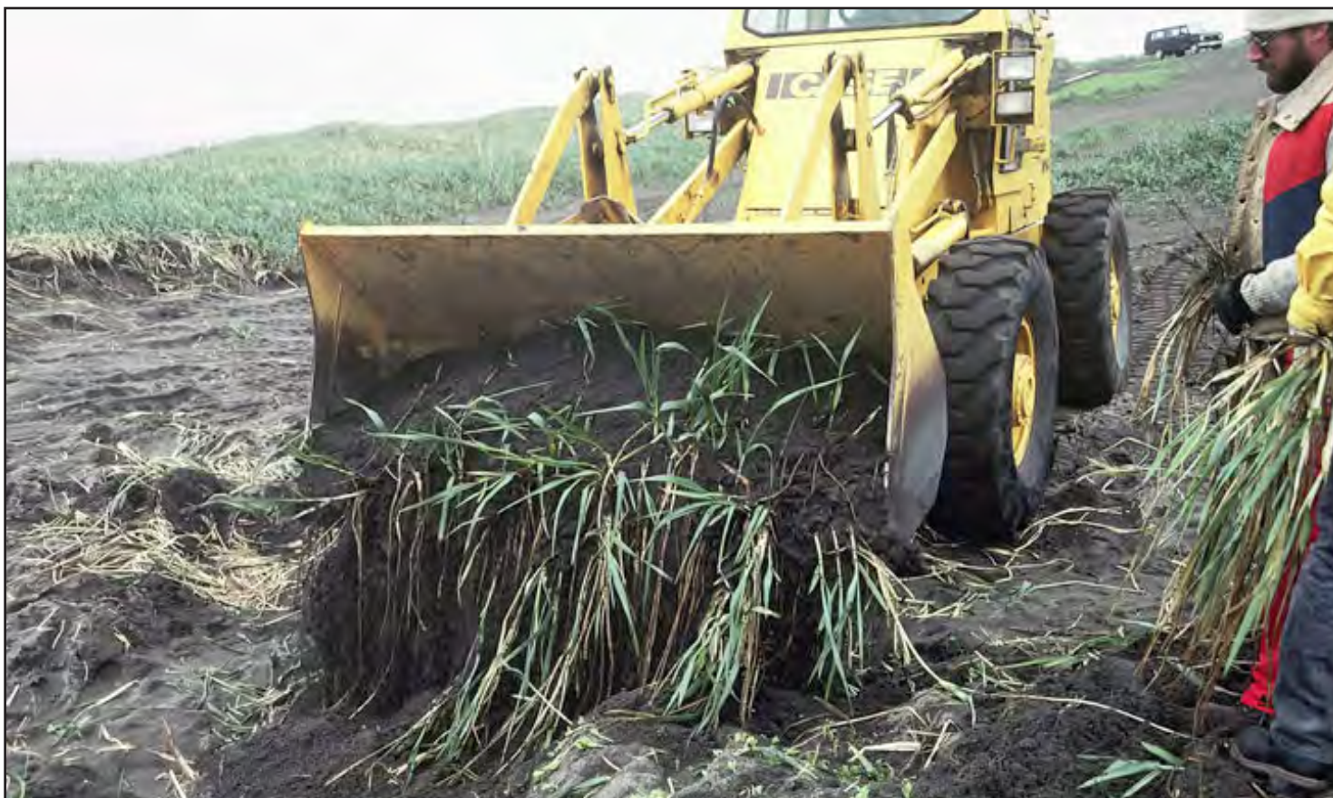
FIGURE a.10: Loader used to harvest sprigs
