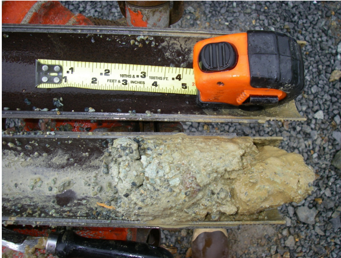
Example of silty gravel (Borehole G10-BH01, Sample 5, 30.0 to 31.5 feet depth).
