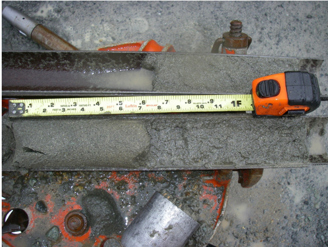
Example of poorly graded “beach sand” (Borehole G10-BH04, Sample 6, 20 to 21.5 ft depth).
