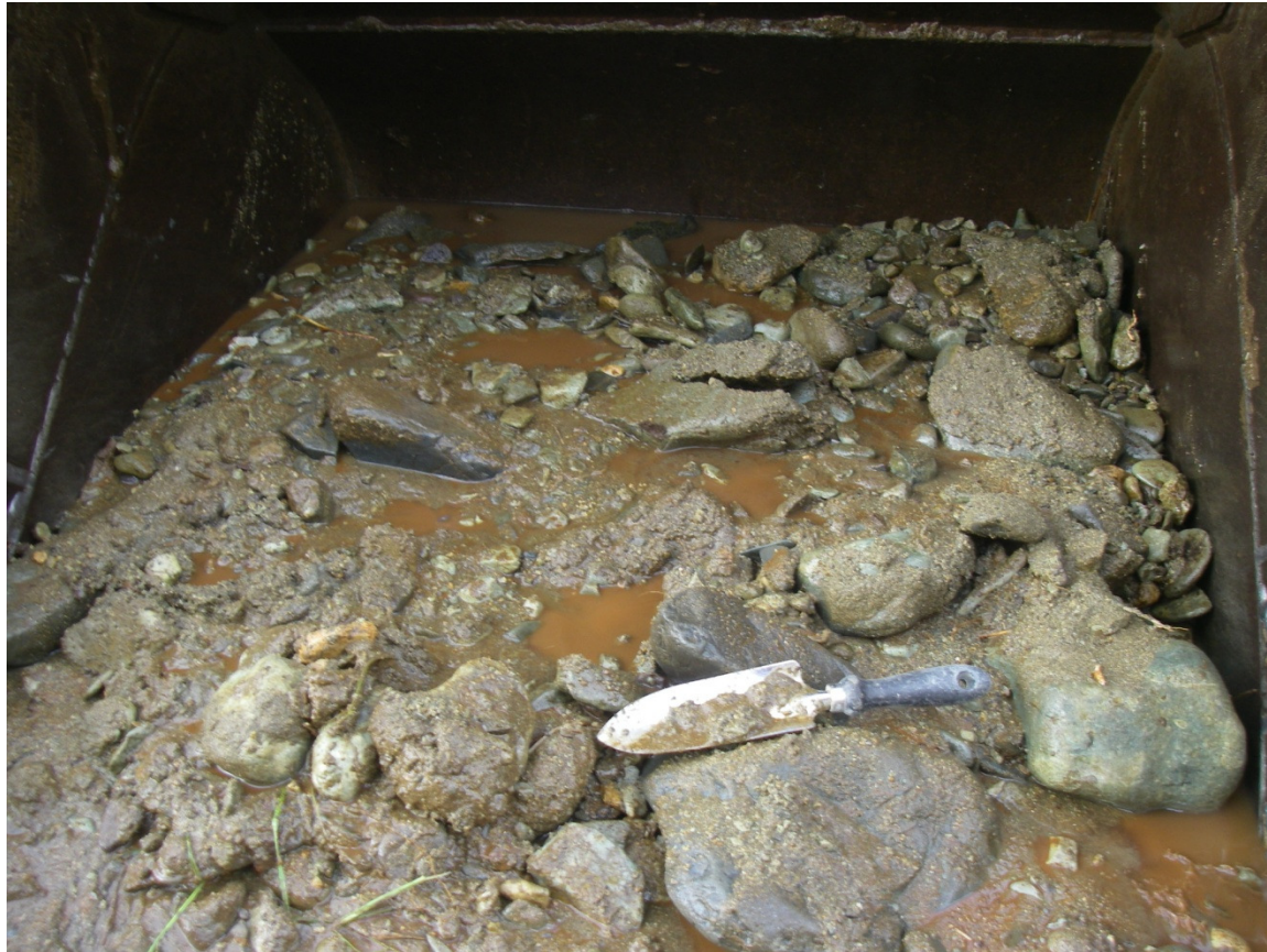
Example of poorly graded “beach cobbles and gravel” (Test Pit G10-TP06, Sample 3, 7 to 9 feet depth). Trowel is approximately 0.9 feet long.
