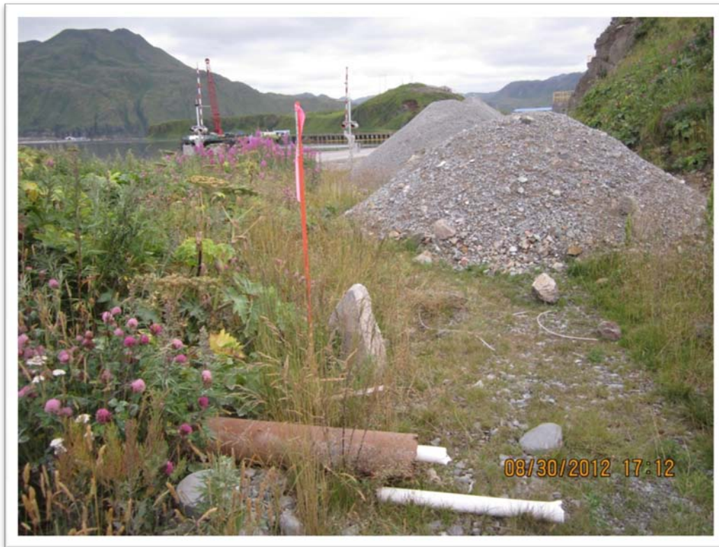
Photograph 1 – Well MW-1 was destroyed. View to the southeast.
