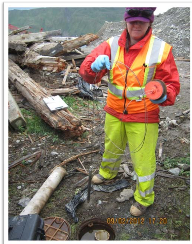
Photograph 14 – Installing transducer in MW-10, view to the south.
