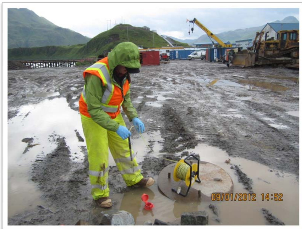
Photograph 16 – Collecting a water level measurement at well MW-11. A tall cap was installed over well due to surface water ponding, when survey was conducted for this well the elevation measured was to the top of the cap.
