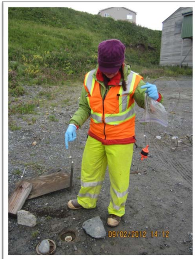
Photograph 10 – Installing transducer in well MW-7R, view to the north.
