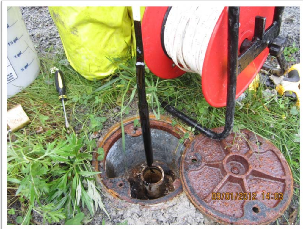
Photograph 27 – Water level could not be obtained in MW-19 due to viscous product completely coating the probe. Depth to product was measured at approximately 12 feet.
