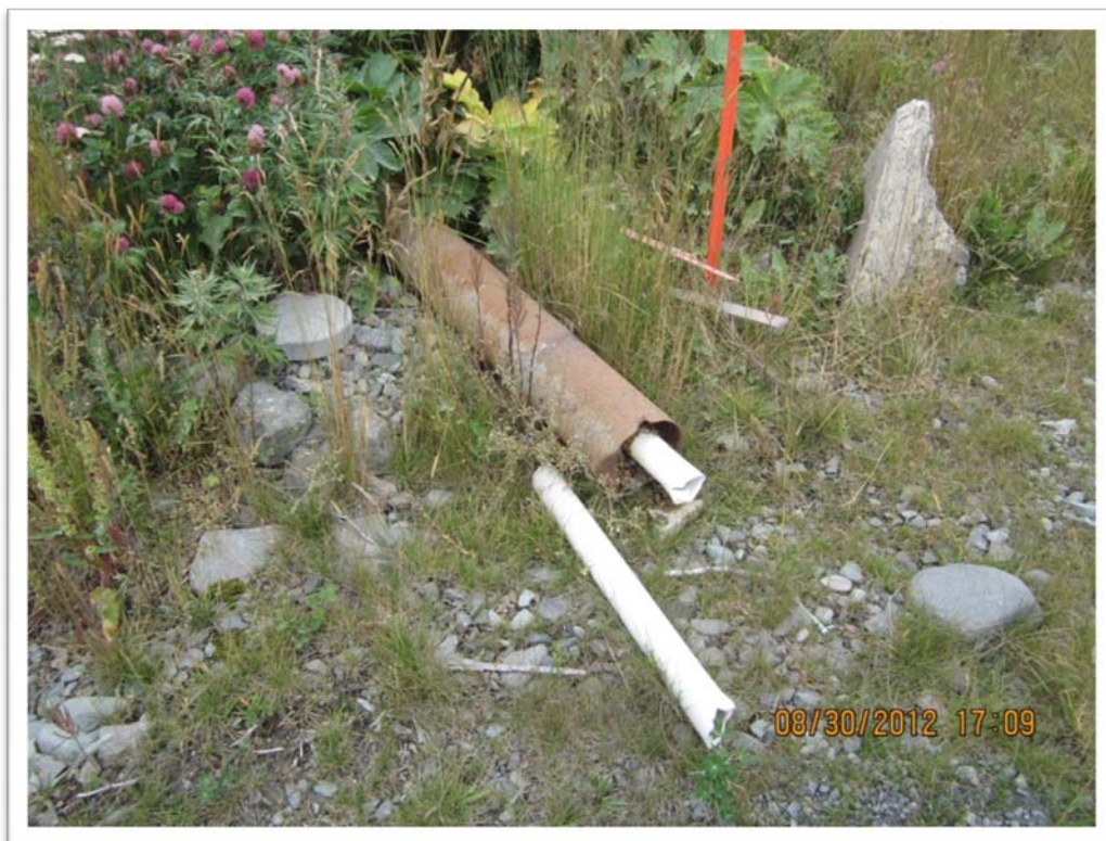
Photograph 2 – Well casing and monument for destroyed MW-1.
