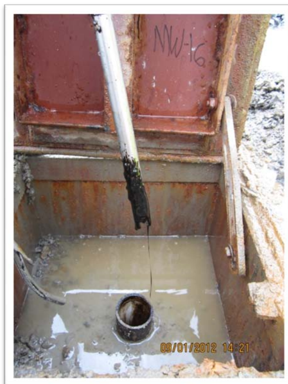
Photograph 20 – Discovering product while attempting to measure water level at MW-16N. Product was detected at approximately 6.55 feet (with a thickness of 0.01 feet) and again at 15 feet near the bottom of the water column (total depth in well was 16 feet).
