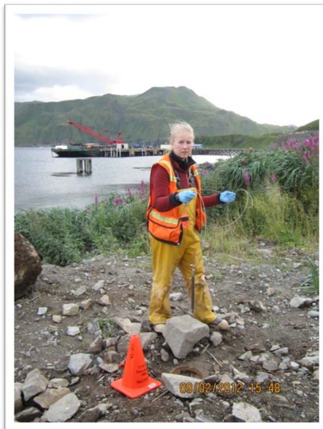
Photograph 29 – Installing transducer in well MW-22, view to the southeast.
