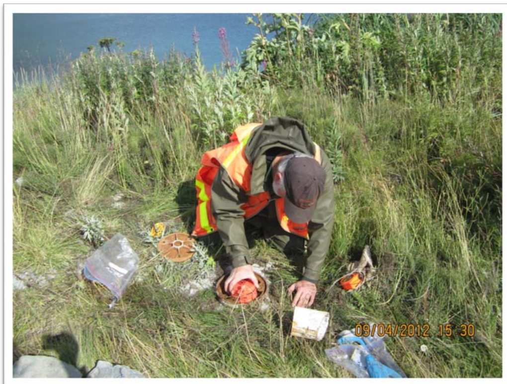
Photograph 18 – Installing transducer and locking cap on well MW-15, piece of PVC cut to accommodate locking cap is visible in center of photograph. View to the east.
