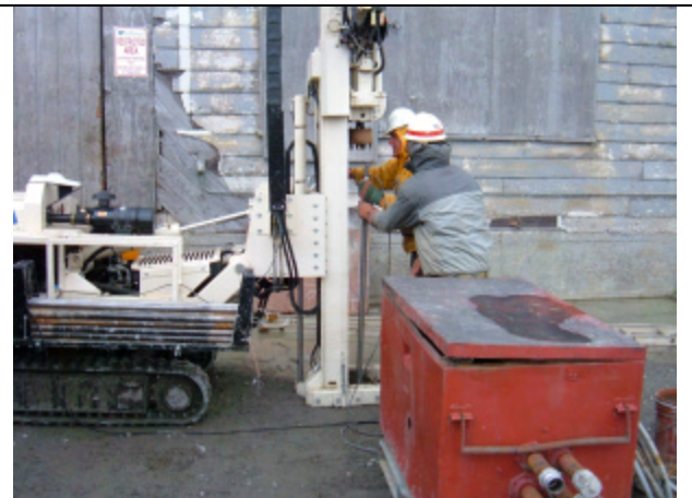
Performing ROST work at Area 2 (LIF point AMK 069)
