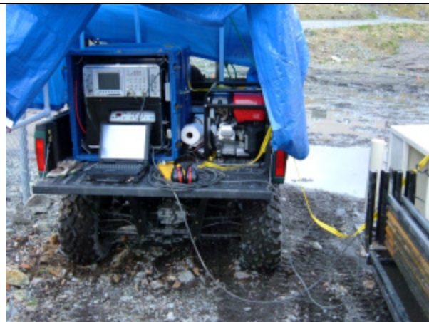
Support vehicle with ROST and generator
