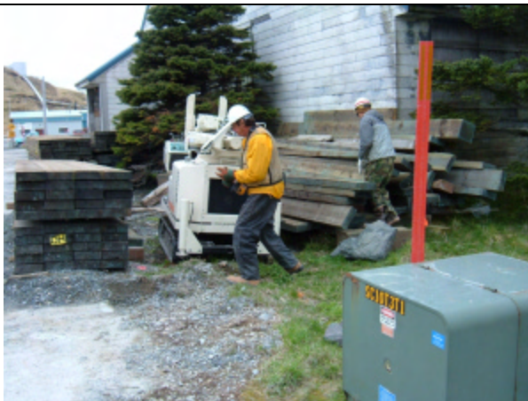
Performing ROST work at suspected bunker C boundary (LIF point AMK 064)
