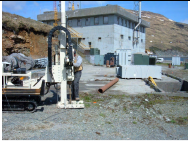
Performing ROST work at Area 1 (LIF point AMK 017c)
