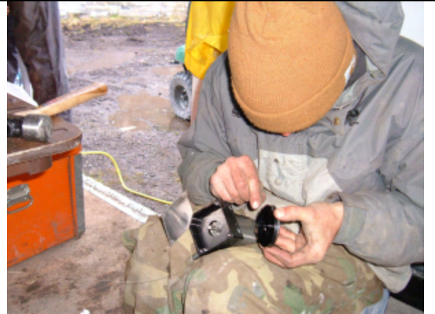
Attempting to repair damaged string pot
