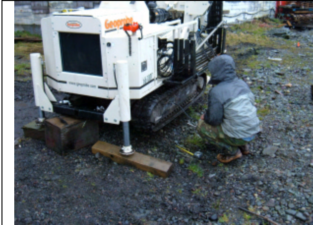
Repairing idler wheel and tightening track on drill rig
