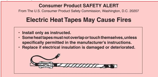
Electric heat tapes are used by thousands of homeowners (especially mobile homeowners) to protect their water pipes from freezing. Yet, if improperly installed or maintained, heat tapes could go beyond keeping your pipes warm; they could burn your house down.
