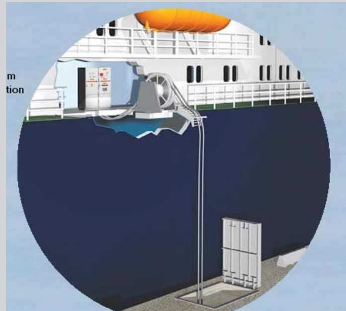
Shore-to-Ship Power System (image courtesy of ABB)
