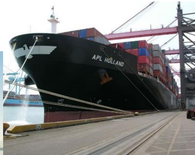
Figures: APL Holland, example container ship that calls on Dutch Harbor. Design vessel static design draft of 44.0 feet
