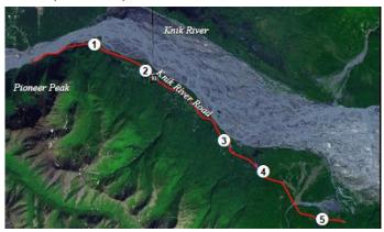
(1) Bingham Hill (MP 1.9) Reconstruct the horizontal curve to correct insufficient superelevation. Widening the shoulder and side slopes provided adequate clear zone width. The design required careful evaluation of the shallow bedrock below the road and along the side slopes.
