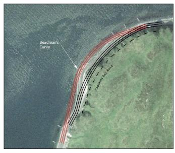
As discussed previously, the realignment may consist of cutting back the slopes or filling on the ocean side. The conceptual sketch above depicts two options at Deadman's Curve that meet the desired 40 mph rating.
